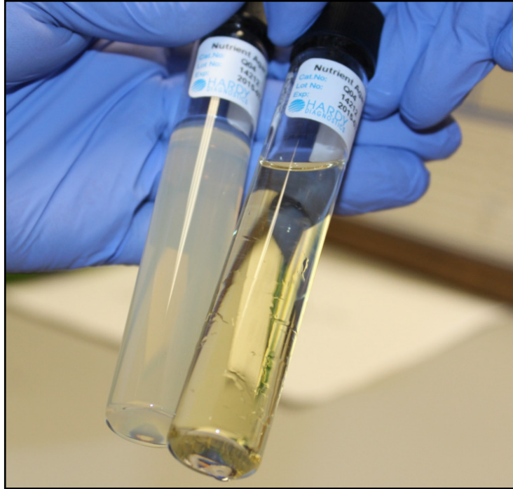
Figure 5. Melted agar is in liquid form on right and is “translucent” while the solid agar on the left is “cloudy”.
