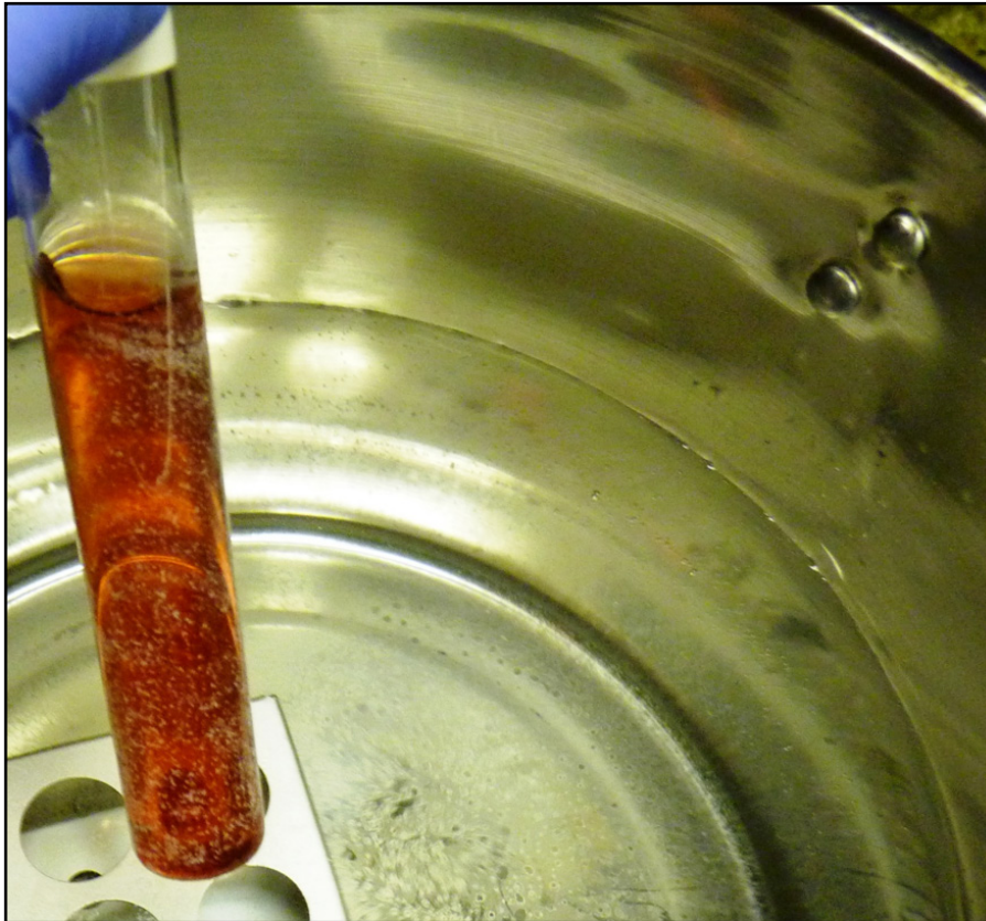
Figure 4. Carefully lifting the agar tubes from the hot water to monitor the melting process.
